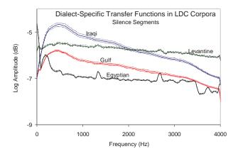
Figure 1: Arabic dialect-specific channel characteristics in LDC corpora estimated as long-term averages of log amplitude spectra in silence segments. Dashed lines – intervals of  $\pm 5\sigma$ .
