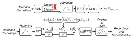
Figure 2: Block scheme of channel estimation, normalization, and signal reconstruction in time domain.
