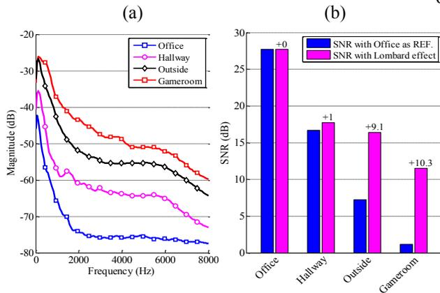
**Figure 2:** (a) Spectral characteristic of real-world maskers using the long-term averaged spectrum. (b) Evaluation of subject's listening environment using the signal-to-noise ratios (SNR) with and without Lombard effect respectively.
