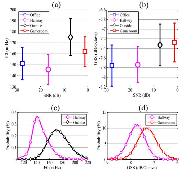
**Figure 3:** Acoustic analysis of speech production: Upper panel is the variation of the speech parameters, (a) fundamental frequency (F0) and (b) glottal spectral slope (GSS), as a function of varying SNR levels. Lower panel is the probability distributions of each parameter for the two most separated conditions.
