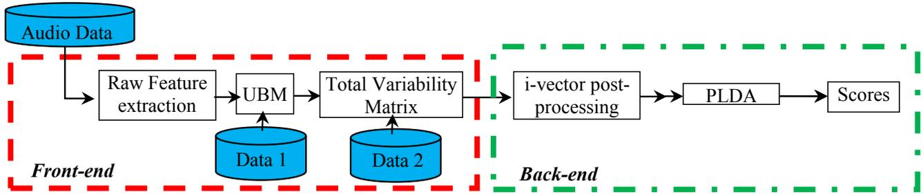
**Fig. 1.** System block diagram of i-Vector based SID for Lombard speech. Data 1 and 2 correspond to raw features for UBM and TV matrix, respectively. Here, both are the same as training data. ‘Audio data’ reflects all acoustic data used in verification.
