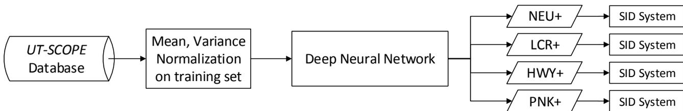
**Fig. 2.** System level block diagram of Deep Neural Network interface with SID systems ('+' indicates presence of non-target speech types in test data).
