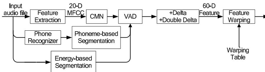
Fig. 2. A block diagram of the feature extraction block of the CRSS systems.
