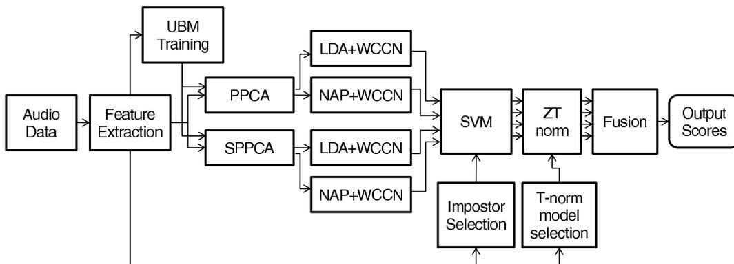
Fig. 1. A conceptual block diagram of the CRSS core system submissions. This shows a fusion of four of our SVM based sub-systems.
