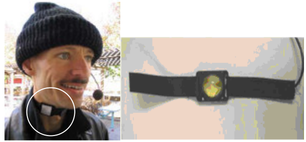
Fig. 3: The Physiological Microphone (PMIC) and its placement around neck
