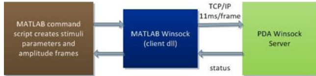
Fig. 8. Device connectivity and data exchange in an offline mode.
