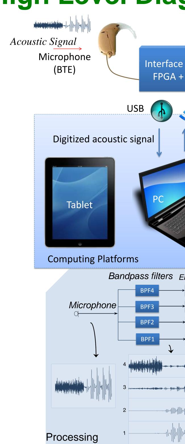
The acoustic signal is first acquired from the BTE and is sampled digitally by an on-board stereo codec and sent to the smartphone wirelessly over Wi-Fi for subsequent processing.
