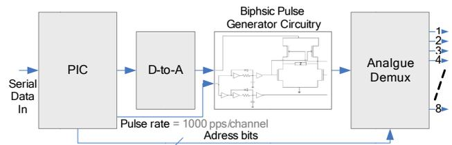
Fig. 6. Logic and stimulator block diagram
