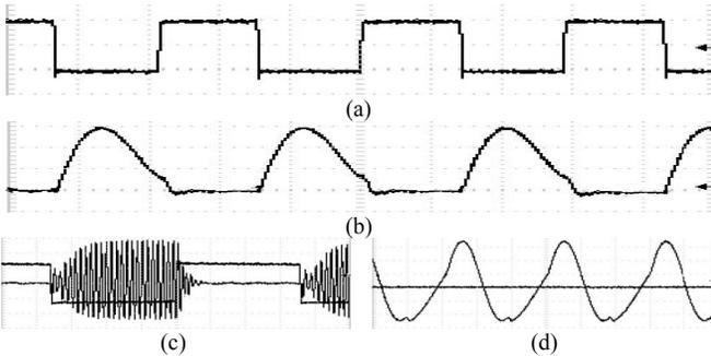
Fig. 9. Class E Waveforms. (a)  $V_{gate}$  (b) drain to source voltage  $V_{DS}$  (c) Data signal at the gate (x6) and voltage across primary coil (d) Voltage across primary coil in high state =  $40 V_{pp}$ , time scale =  $1.4\mu s$
