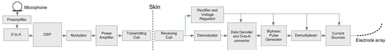
Fig. 1. Block diagram of complete Cochlear Implant system
