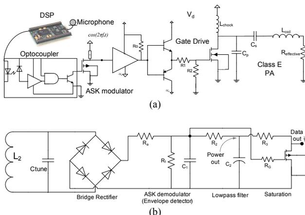
Fig. 5. (a) Transmitter Design; (b) Receiver Design
