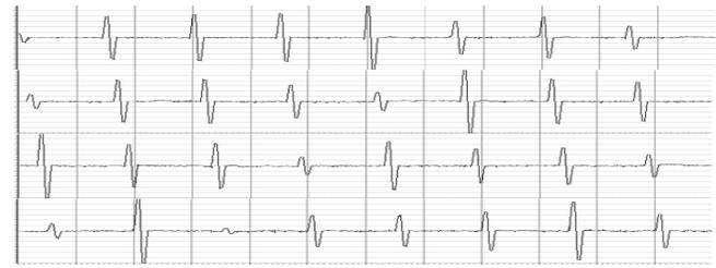
Fig. 11. Interleaved biphasic electrical pulses of the first four channels
