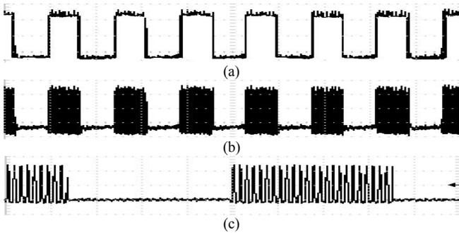
Fig. 8. Voltage Waveforms of the modulating transistor (a) Gate Signal, (b) ASK modulated signal at drain, (c) close view of the ASK modulated signal
