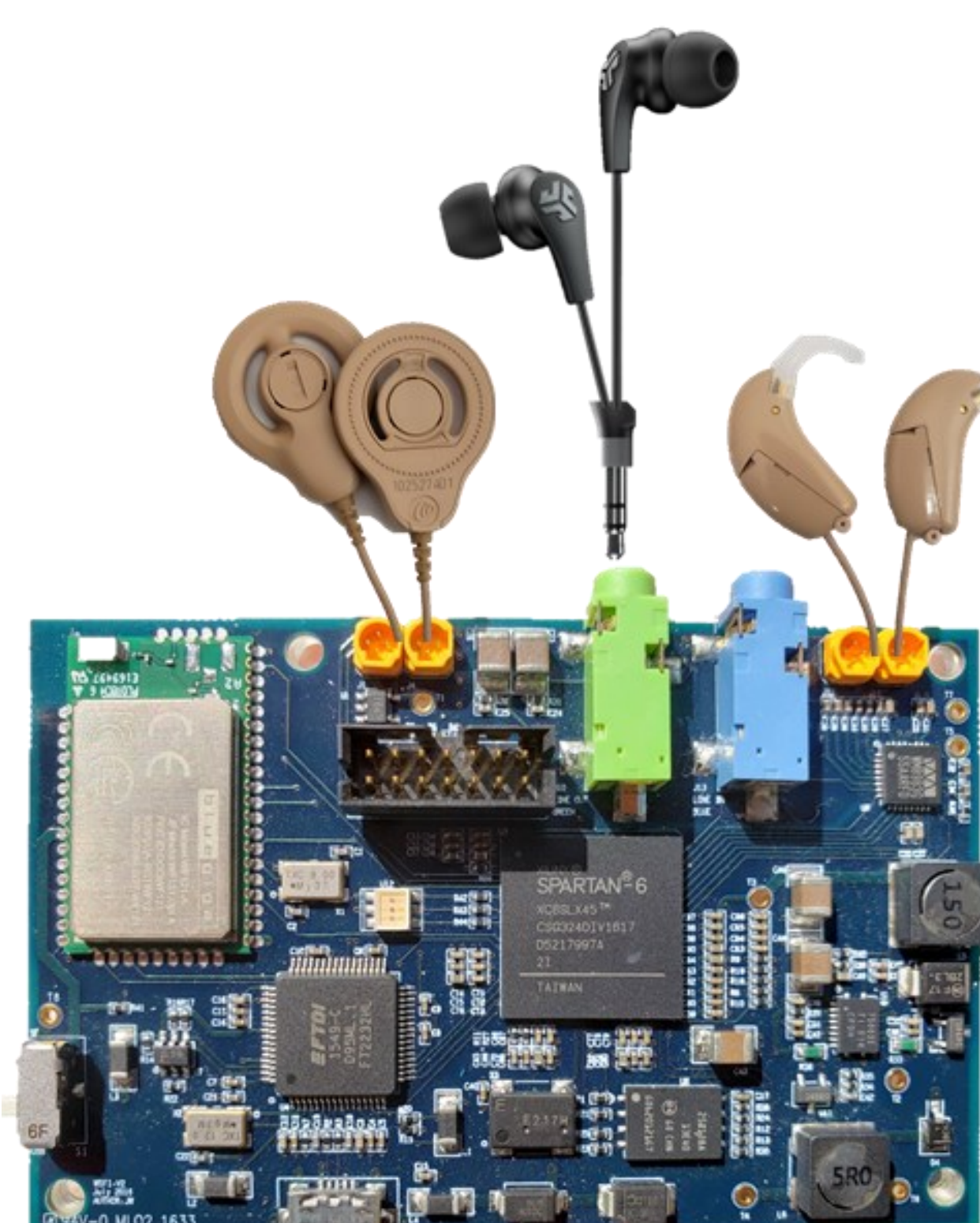
Fig 1. Hardware design and overview of CCI-MOBILE Research Platform.
