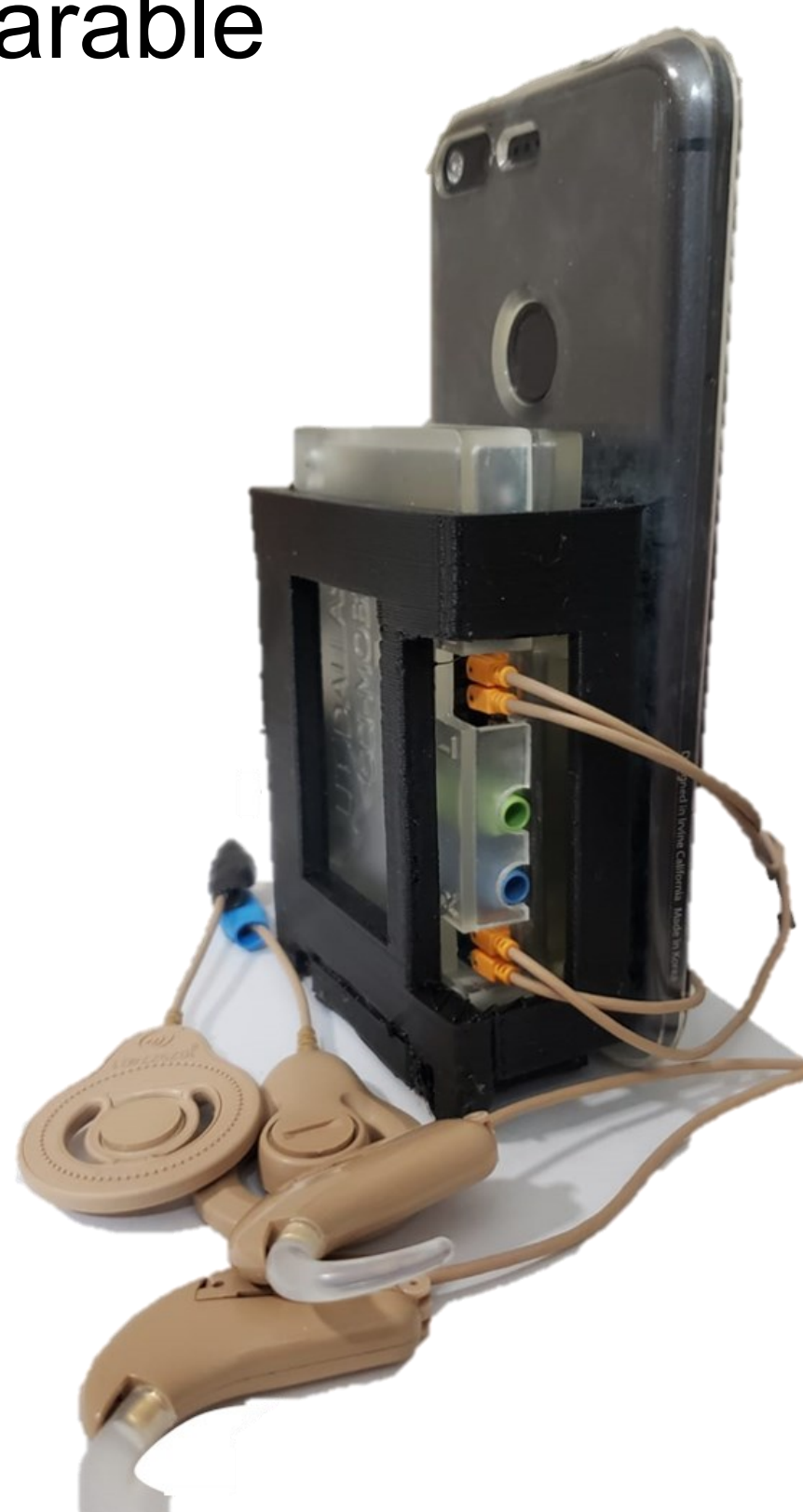
Fig 2. In-field configuration with CCI-MOBILE and Android phone.
