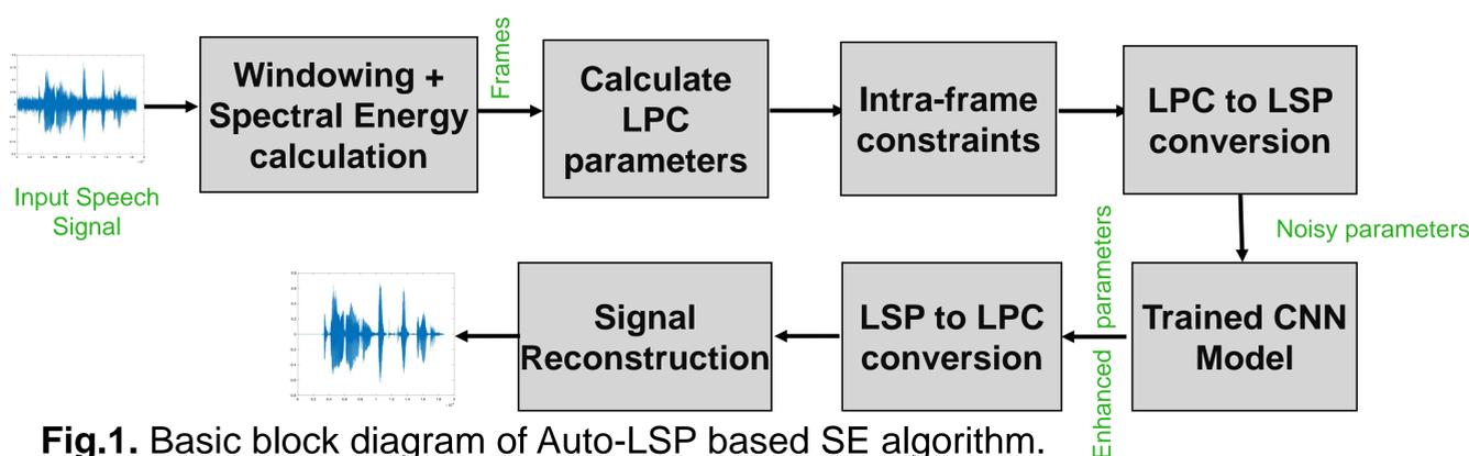
Fig.1. Basic block diagram of Auto-LSP based SE algorithm.
