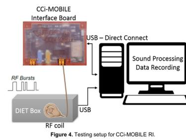
**Figure 4.** Testing setup for CCI-MOBILE RI.
