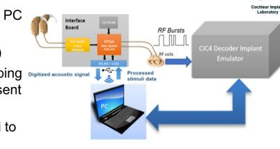
**Figure 5.** Functional block diagram for testing and evaluation.
