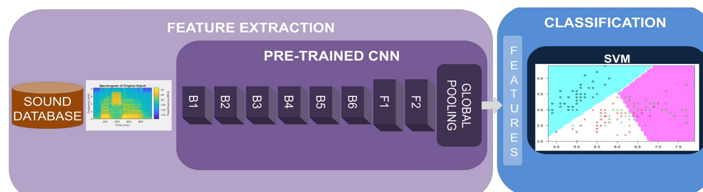
Fig. 2. Framework for sound classification using pre-trained CNN and SVM classifier.
