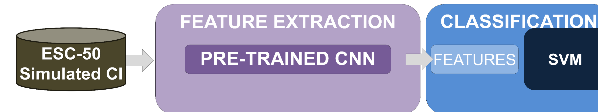
Fig. 4. Sound classification framework in simulated CI conditions for NH listeners.
